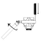
2.Place the microphone on the shock mount with the logo facing the front. Secure the microphone in place by tightening the knob beneath
